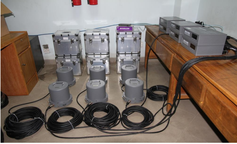
Testing of the broadband seismometers for new six stations
